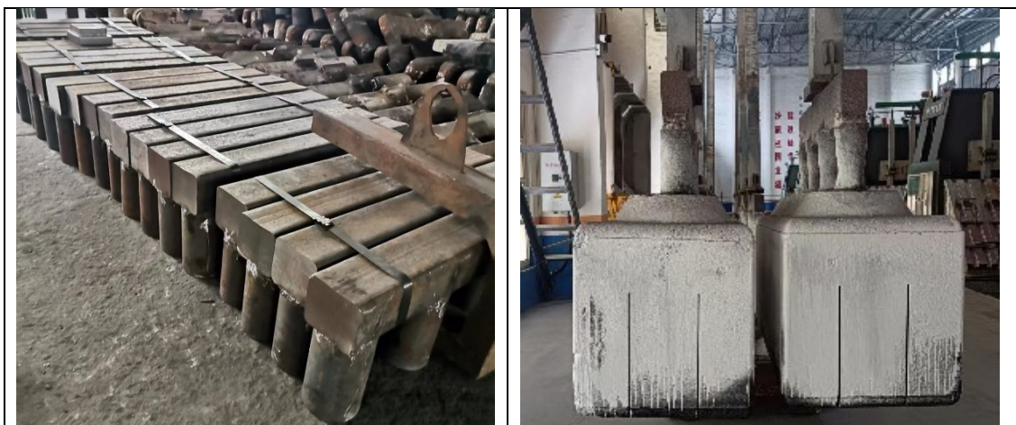
Figure 6. Low resistance anode steel stubs (left). Carbon dust-free slotted anodes (right).
